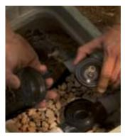
competition. Just one example is the threaded bonnet design that eliminates the need to remove and replace multiple screws to access and maintain the unit. Additional value-added features include:
